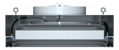
**Step 4:** Scan the filter and diffuser casing to verify overall unit integrity. If leakage in excess of the approved limit is detected, follow the diffuser and filter vendor's recommendations for troubleshooting and field repairs if needed.
